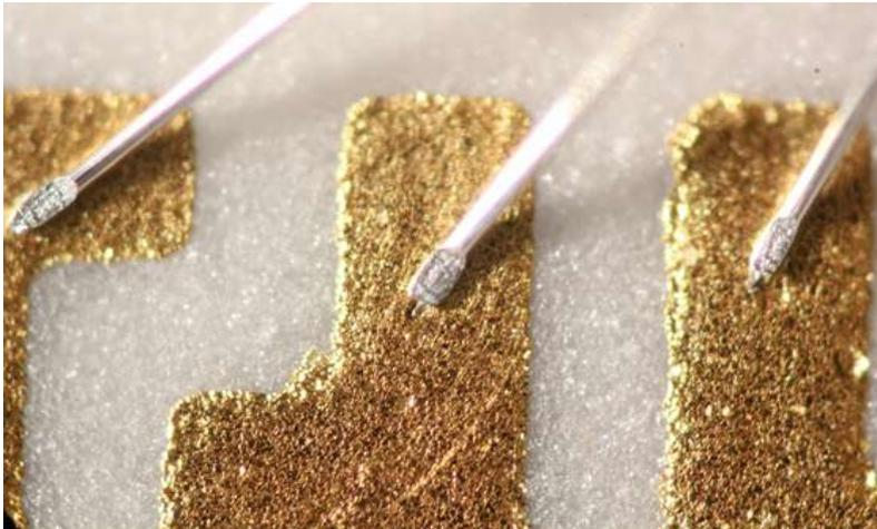
The very small bond wires are attached to the golden circuit paths of the hybrid module. The other end is connected to the silicon dies.
