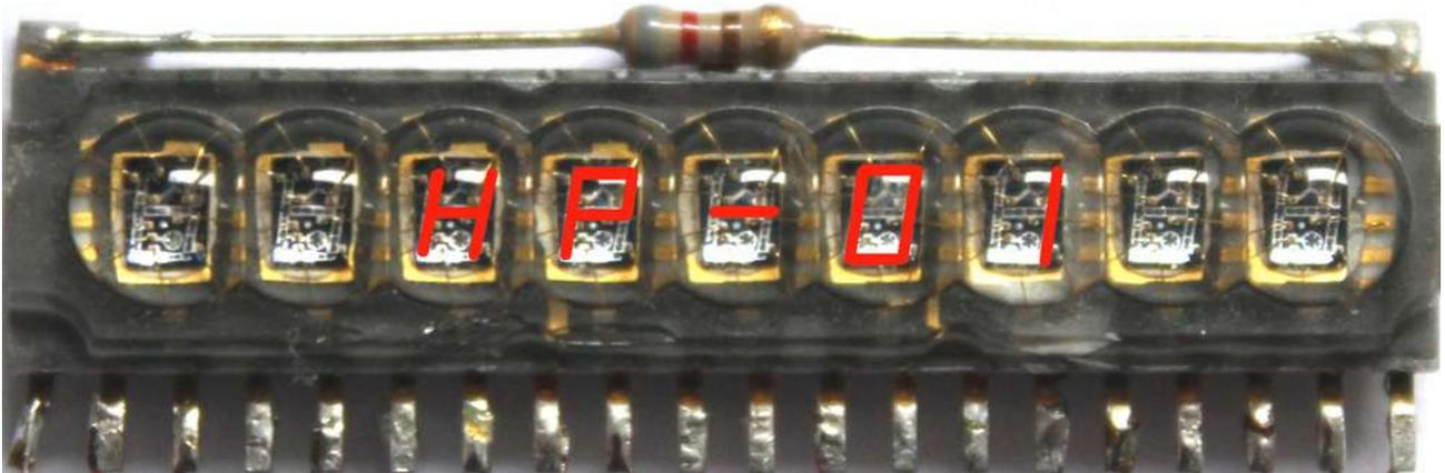
When displaying different digits, some need more current than others. The digit “8” for example has all segments on, and the digit “1” only 2 segments or a single dot with only one segment, will be displayed in different brightness, because the same current flows through 7 segments, or through only 1 or 2 segments. This effect is clearly visible and cannot be tolerated.
