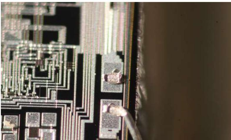
In the middle of the image you can clearly see the empty pad, where the bond wire originally was attached.
