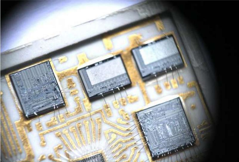
The HP-01 hybrid module with the two ROM chips visible on the upper right.
